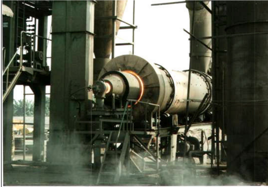
Figure 12. Aggregate being dried by heating in the dryer
