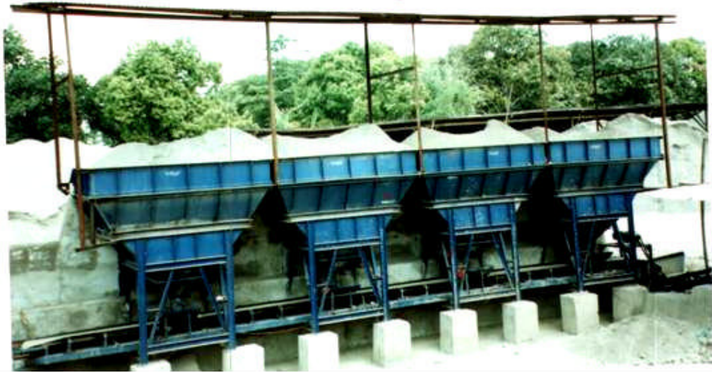
Figure 10. Each Aggregate fraction inside its own bin (cold bin)
