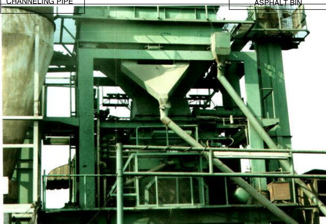
Figure 1. The component on the left is an elevator for buton granular asphalt (filler)
