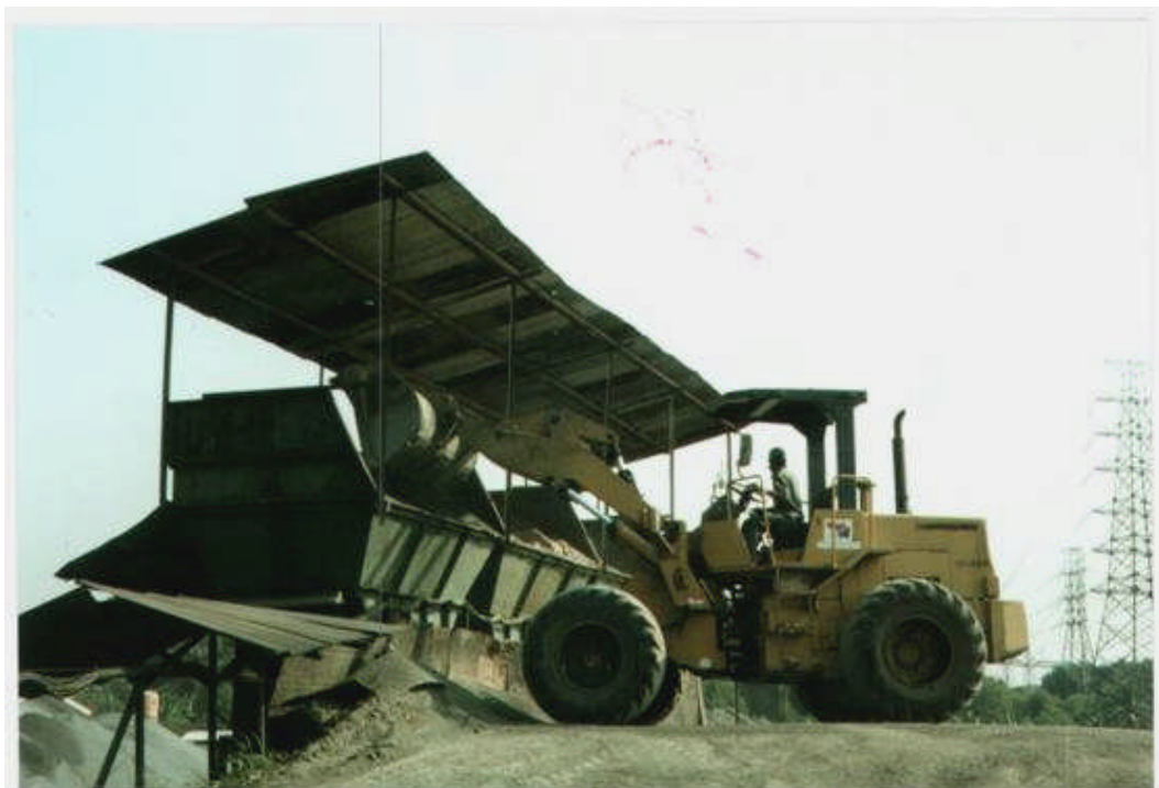
Figure 11. Preparation of loading Aggregate into the Cold Bin by using a wheel loader
